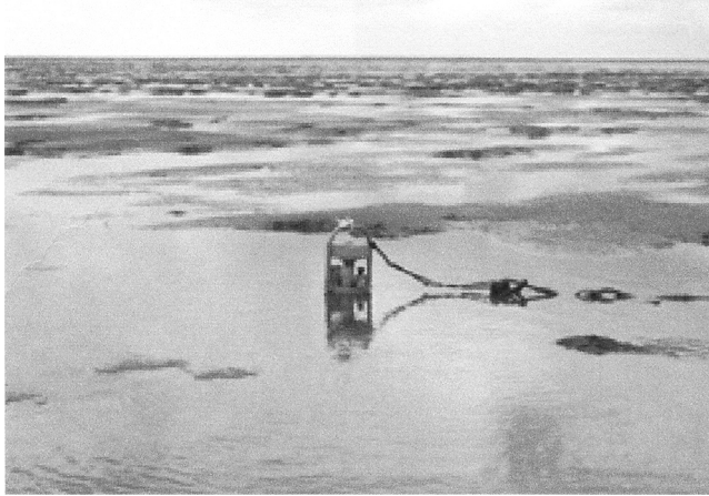
Figure 5. The Aanderaa current meter (RCM 9) placed about two meters from the frame.
